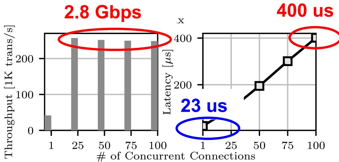
Server has Xeon 2640v4 2.4 Ghz (uses only 1 core) and Intel X540 10 GbE NIC
