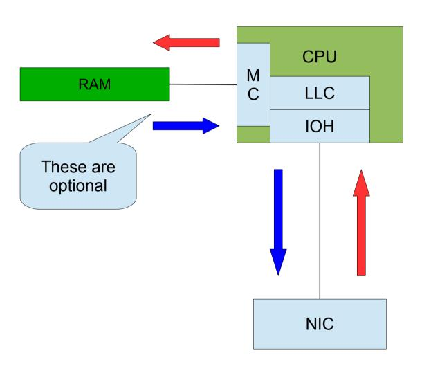
Red = DMA Request Blue = DMA Reply
