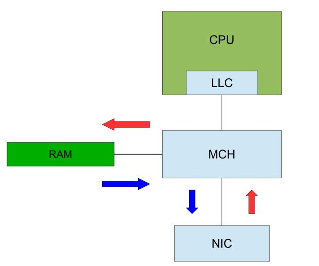
Red = DMA Request Blue = DMA Reply
