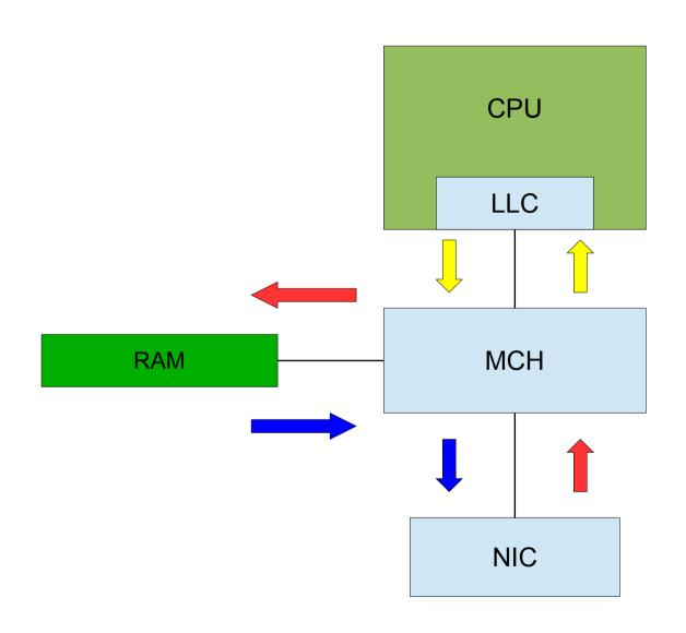
Red = DMA Request Blue = DMA Reply Yellow = Snooping
